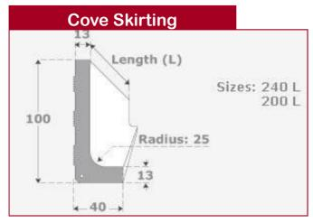
Available in 240 and 200 Long. Easily mitre -cut on site to form internal and external corners
